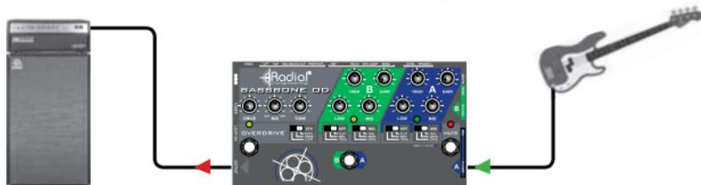
Start by testing the audio to make sure everything is working. Increase the GAIN on channel-A to about the 2 o'clock position. Slowly turn up the volume on your bass amp. It is a good practice to test at a low volume level should a faulty cable or other problem be encountered.
