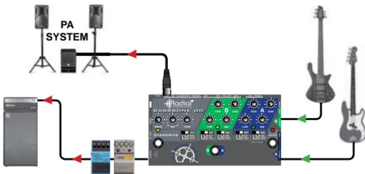
To take things one step further, the Bassbone OD is equipped with an effects loop. When pedals are connected in the loop you can use them with both instruments and choose to send the pre-effects signal (dry) or the post-effect signal (wet) to the PA.
