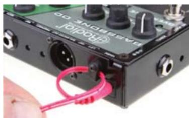
Connect your electric bass to INPUT-A. Connect the 1/4" OUTPUT jack to your bass amp. The A/B select switch toggles your bass between channel-A and channel-B. Make sure channel-A is selected, the green LED will illuminate.
