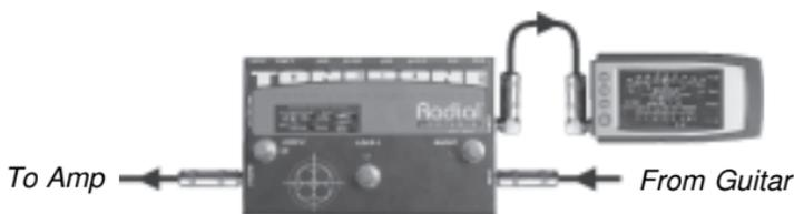
*Tuner output is always on for 'on the fly' tuning*
